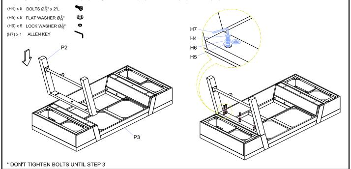
Step 2: Attach metal stretcher (P4) to right leg (P2) using Lock washer (H3), Flat washer (H2) and Bolt (H1) as shown below.
